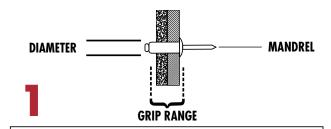
SELECT RIVET WITH GRIP RANGE LARGER THAN THICKNESS OF MATERIALS TO BE FASTENED.
