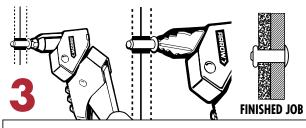
PLACE RIVET IN HOLE. SQUEEZE HANDLE TO PULL & CUT OFF EXCESS MANDREL (YOU MAY HAVE TO SQUEEZE MULTIPLE TIMES).
